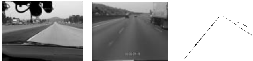
Fig. 3: These figures show the view showing the mounted cameras and performance of the lane extraction system on a typical input image.
