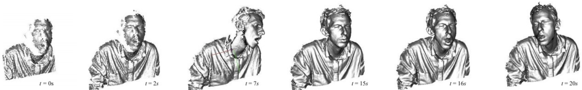
Figure 1: Real-time reconstructions of a moving scene with DynamicFusion; both the person and the camera are moving. The initially noisy and incomplete model is progressively denoised and completed over time (left to right).
