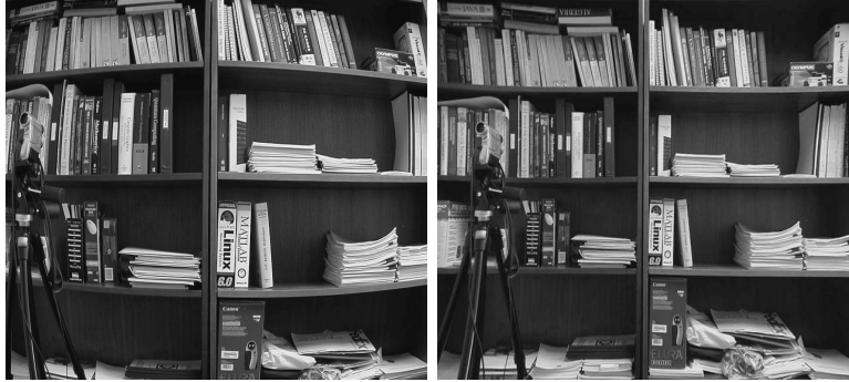
Figure 3.9. Left: image taken by a camera with a short focal length; note that the straight lines in the scene become curved on the image. Right: image with radial distortion compensated for.
