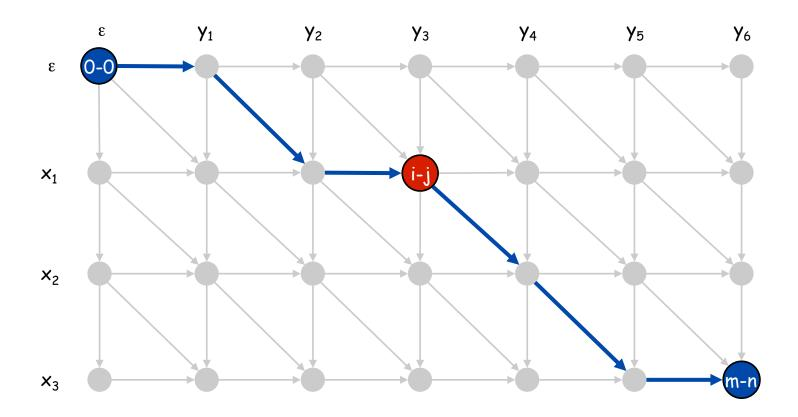
Observation 2. let q be an index that minimizes f(q, n/2) + g(q, n/2). Then, the shortest path from (0, 0) to (m, n) uses (q, n/2).
