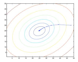
The ellipses shown above are the contours of a quadratic function. Also shown is the trajectory taken by gradient descent, with was initialized at (48,30). The x's in the figure (joined by straight lines) mark the successive values of  $\theta$  that gradient descent went through.
