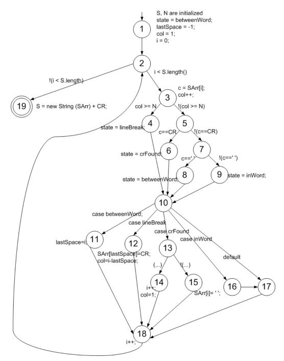
Note that in the switch statement, there is a separate node for the case inWord, which, due to Java semantics, falls through directly to the default case.
