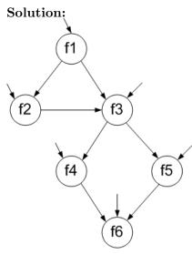
Note that in the call graph, all of the **public** methods are potentially initial nodes. Final nodes are not marked in the given diagram. However, the code shown suggests that  $f^2$  is final (since there is no requirement that further calls are made), and that  $f^6$  may be final (no calls are shown). The remaining nodes are not final; there is always another call from  $f^1$ ,  $f^3$ ,  $f^4$ , and  $f^5$ .
