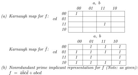
f = abca + abcaNonredundant prime implicant representation for  $\bar{f}$ :  $\bar{f} = a\bar{b} + b\bar{c} + c\bar{d} + \bar{a}d$
