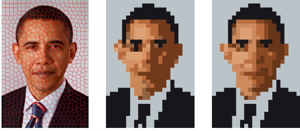
Figure 6: Without the Laplacian smoothing step, the superpixels (left) tend to have 6-connected neighborhoods. This causes small distortions in the output (center), which are particularly noticeable on the ear, eye and mouth, when compared to original output that uses the superpixels that included the smoothing step (right).
