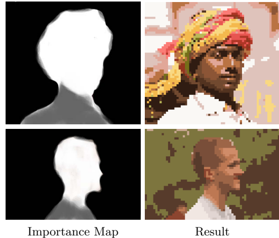
772 Figure 15: Results using an importance map. (top) 64 \times 58 , 773 16 colors (bottom) 64 \times 43 , 12 colors
