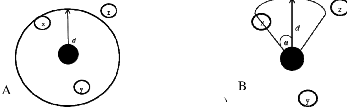
Fig. 2. Sense pre-processing areas A) \alpha is 360 degrees around the agent. In this example, x and y are sensed by the agent, but z is not. B) \alpha is less than 360 degrees. In this example, only object x is sensed.
