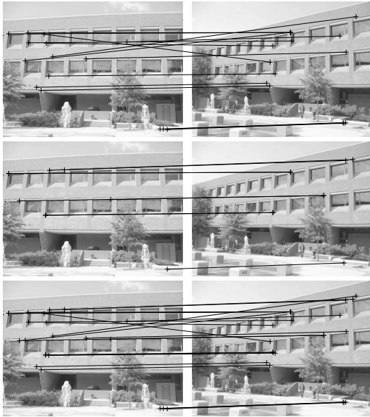
Figure 5: (left) Match result using only Lowe's criteria (15 matches); (center) result using only cosine measure (9 matches); (right) result using both measure(22 matches).
