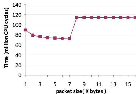
Figure 3: Network overhead for variable packet size.
