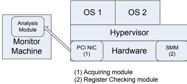
Figure 2: The architecture of HyperCheck
