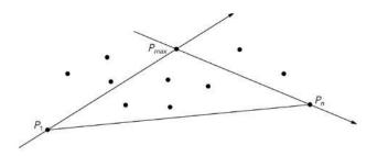
Algorithm 4.4 takes a line and a set of point. The points are all on the same side of the line. Then a triangle is formed by the line and the furthest point from the line. All points inside the triangle are removed. The remaining points are divided into two groups. (why is it two groups? why not three?) Algorithm 4.4 is called recursively until no points remain.
