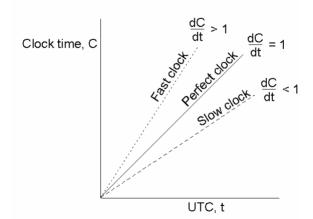
The relation between clock time and UTC when clocks tick at different rates.
