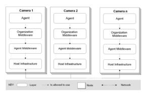
Figure 1. Deployment view of the traffic monitoring system.
