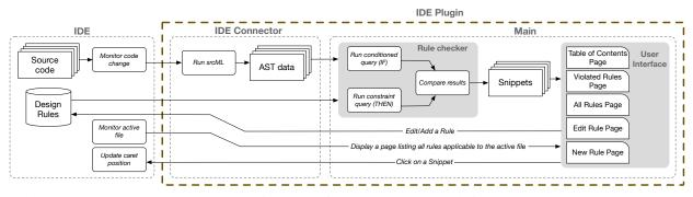
Fig. 8: The ACTIVEDOCUMENTATION system architecture. After a source code or design rule change, srcML generates an AST in an XML format. The rule checker then verifies each design rule against the AST by running two XPath queries, one for the quantifier and one for the constraint, generating a list of matches for each query. These matches are compared, generating a list of design rule examples and violations. These are then displayed to the user in several pages.
