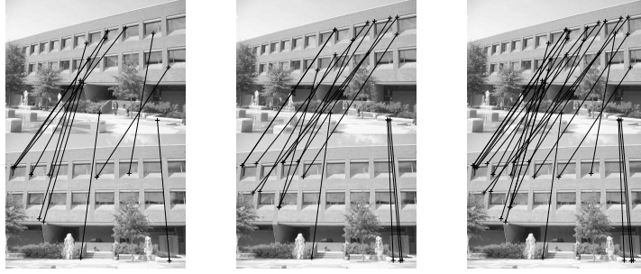
Fig. 4. Matches obtained using: distance ratio (left, 11 matches); cosine measure (middle, 15 matches); combining both measures (right, 24 matches).
