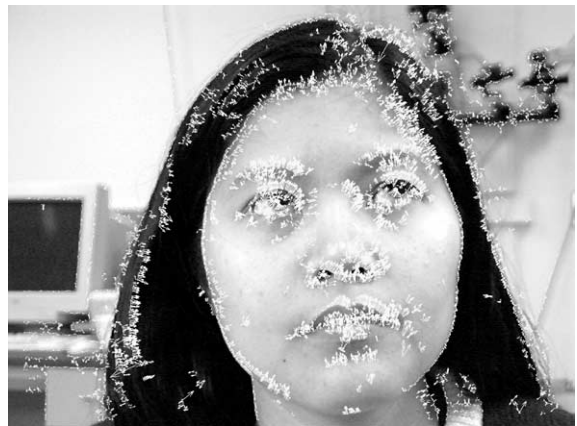
Fig. 8. Normal flow displayed as vectors emanating from the edges found in one of the frames shown in Fig. 1.
