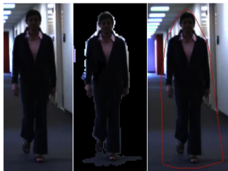
frames, foreground, convex hull
