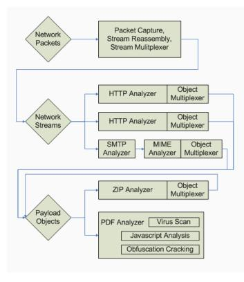
Figure 1: Rumiante Components
