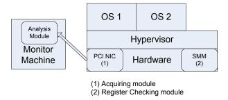
Figure 2: The architecture of HyperCheck
