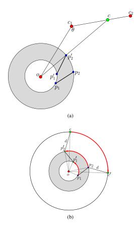
Figure 5: (a) The swept area of  $\overline{p_1p_2}$  rotating is bounded by this grey shadowed donut-shape. The closest distance between  $\overline{p_1p_2}$  and *c* is realized when  $p_2$  becomes colinear with *o* and *c*. (b) If  $\overline{p_1p_2}$  is fixed and *c* rotates around *o* with velocity  $-\omega$ , both the closest features and closest distance will be the same as in the case where *c* is fixed and  $\overline{p_1p_2}$  rotates around *o* with  $\omega$ .
