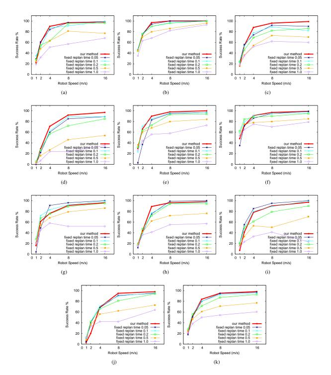
Figure 11: Compare our method to the fixed-time strategy on success rates for environments in Fig. 10. In the fixed-time strategy, the robot replans every 0.05, 0.1, 0.2, 0.5 and 1.0 seconds. For every specific robot velocity, (k) plots the average success rate over all these 10 environments.
