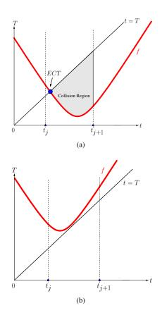
Figure 2: The red (thicker) curves in both figures are plots of the earliest arrival time f(t) for an obstacle. Black straight lines are plots of g(t) : t = T. (a) When there is at least one intersection (blue dot) between f(t) and g(t), **collision region** is not empty. (b) Otherwise, the **collision region** is empty.
