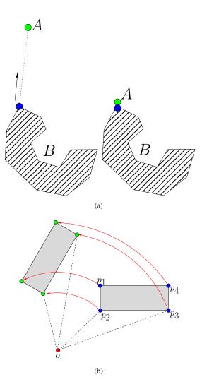
Figure 4: (a) If A is fixed and B translates towards A along the closest direction, the closest features between B and A remain the same until they collide. (b) A polygon rotates around a point o. The area it sweeps over is bounded by the trajectory of every vertex ( $p_1$  through  $p_4$ ) and edges from both original and destination shapes.
