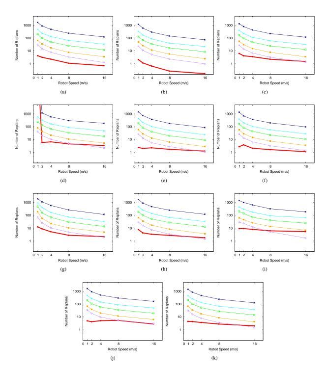
Figure 12: Compare our method to the fixed-time strategy on number of replans for environments in Fig. 10. In the fixed-time strategy, the robot replans every 0.05, 0.1, 0.2, 0.5 and 1.0 seconds. For every specific robot velocity, (k) plots the average number of replans over all these 10 environments. Notice that the *y*-axis of (b) is in logarithmic scale.
