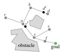
Figure 9: An RRT augmented with earliest collision time. The tree is rooted at current configuration r of the robot. Configurations c' and d' are the predicted earliest collision locations on the paths from r to c and d, respectively.
