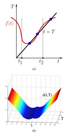
Figure 8: (a) The plot for f(t) when the closest feature to c locates on  $\overline{p_1p_2}^\circ$ . The *collision region* is bounded by the two leftmost intersections. (b) The 3D plot shows the closest distance between an edge of some obstacle and the robot changes over time.
