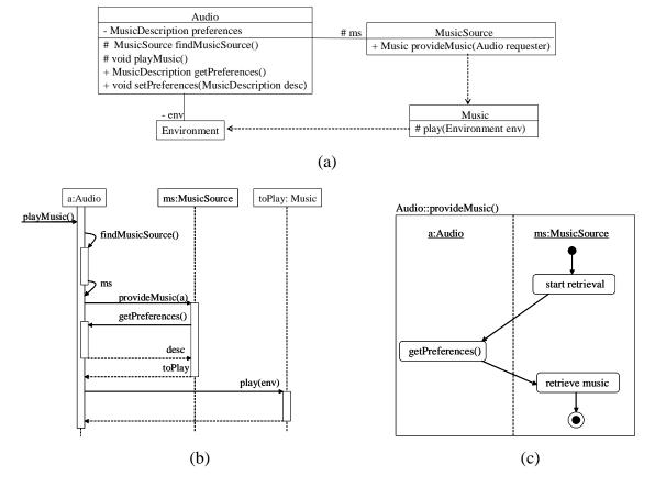
Figure 6. The UML diagrams after variable encapsulation. a) class diagram, b) sequence diagram, c) activity diagram.
