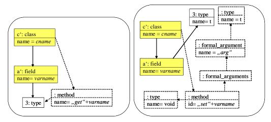
Figure 14. Two NACs for the rule in Figure 13, to check that no method exists with the same signature as the inserted setter and the getter methods.
