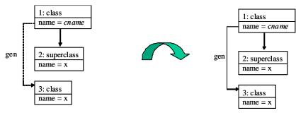
Figure 11. The rule to start the computation of the ancestors of the class named cname.
