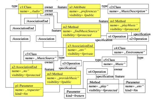
Figure 8. The abstract graph for the class diagram of Figure 5a
