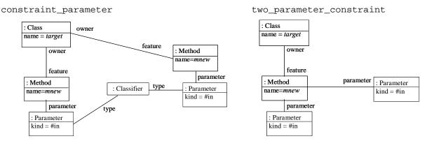
Figure 21. The two graphs to express the constraint for methods with only one parameter.
