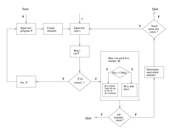
Figure 3: A Mutation Testing Process
