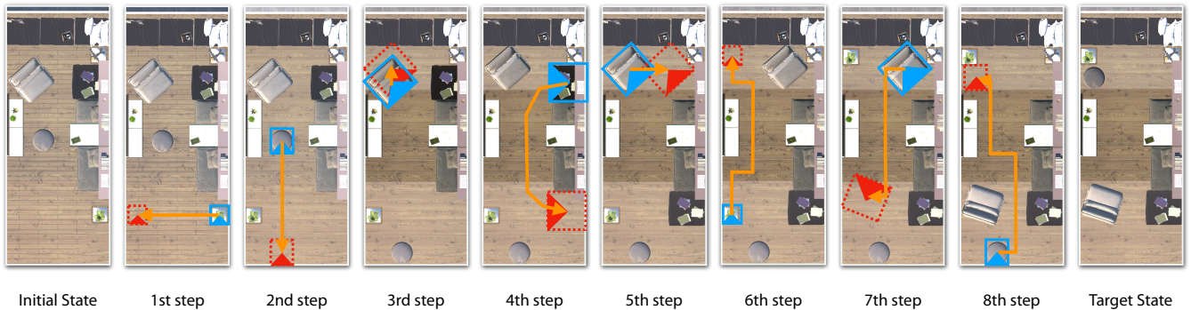
Figure 2: An example of our approach. The bounding boxes represent the position and the orientation of objects. The blue bounding box represents the object to move in this step. The red bounding box with dashed line represents the target position of this object. The orange line represents the moving path.
