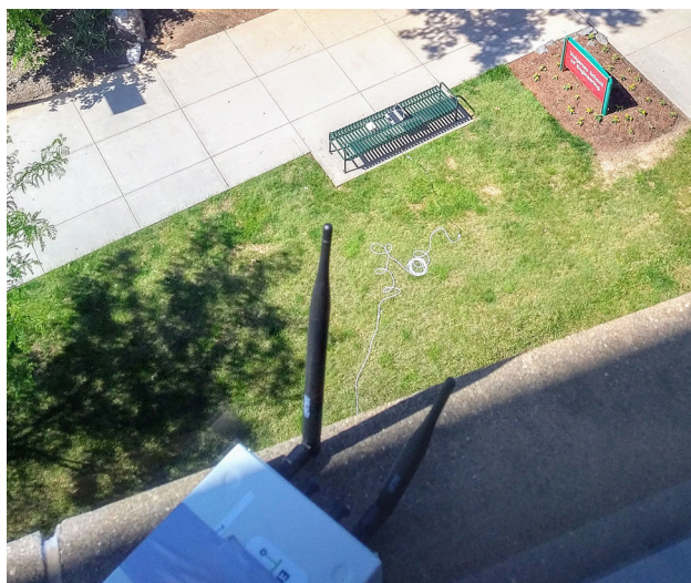
Fig. 19 Test area that was used for elevation tests. Receiver is placed on the ground and the sender is elevated
