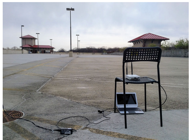
Fig. 12 The test area that was used for distance measurements. Sender and receiver are 100 m apart
