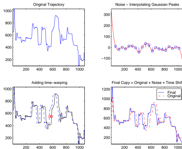
Figure 4: Generation of variations on the heterogeneous data. We produced variations of the original patterns by adding small time warping (2-3% of the series length), and interpolated Gaussian noise. Gaussian noisy peaks are interpolated using splines to create smooth random variations.
