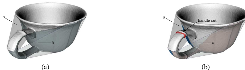
Figure 10: (a) The pocket (shaded area) is enclosed in the projected boundaries of two bridges \beta and \alpha . (b) Pockets after genus reduction.
