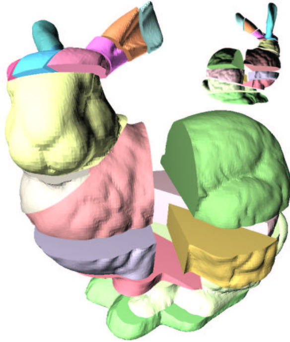
Figure 1: Each component is approximately convex (concavity less than 10 by our measure). There are a total of 17 components.
