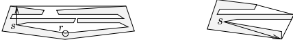
Figure 8. Let r be the notch with maximum concavity. After resolving r , the concavity of s increases. If \text{concave}(r) is less than \tau , s will never be resolved even if \text{concave}(s) is larger than \tau .
