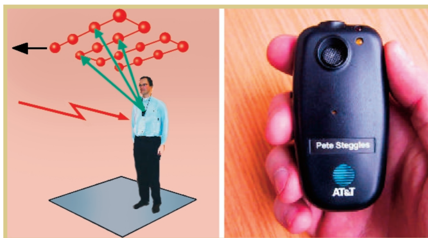
Figure 1. (a) The AT&T Active Bat system and (b) the Bat wireless tag device.
