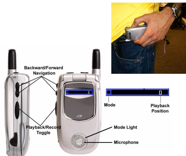
Figure 1 The Personal Audio Loop. Main picture: the device and its interface. Three buttons control record/playback mode and allow to browse the recording. A timeline and a mode light indicate the current operating state. Upper-Right picture: the device can be attached to a belt clip.
