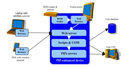
Figure 3. PIP Architecture: Embedded and portable devices use standard Web browsers to connect to the PIP system via Web servers installed on each PIP-enhanced device. PIPs scripts construct the interface using information from a shared database, resources on the user's PC, and features of the PIP-enhanced device.
