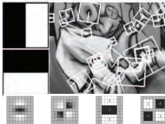
Figure 3.9: The SURF detector and descriptor were designed as an efficient alternative to SIFT. Instead of relying on ideal Gaussian derivatives, their computation is based on simple 2D box filters, which can be efficiently evaluated using integral images. IMAGE SOURCE: Herbert Bay
