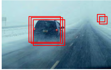
Figure 9.2: Non-maximum suppression is a useful post-processing step to prune out nearby detections.
