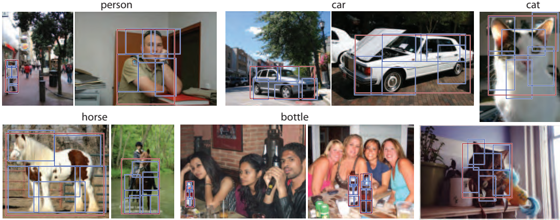
Figure 11.10: DPM recognition results for several categories of the PASCAL dataset (Everingham et al. 2010) (Images from Felzenszwalb, Girshick, McAllester & Ramanan (2010)).
