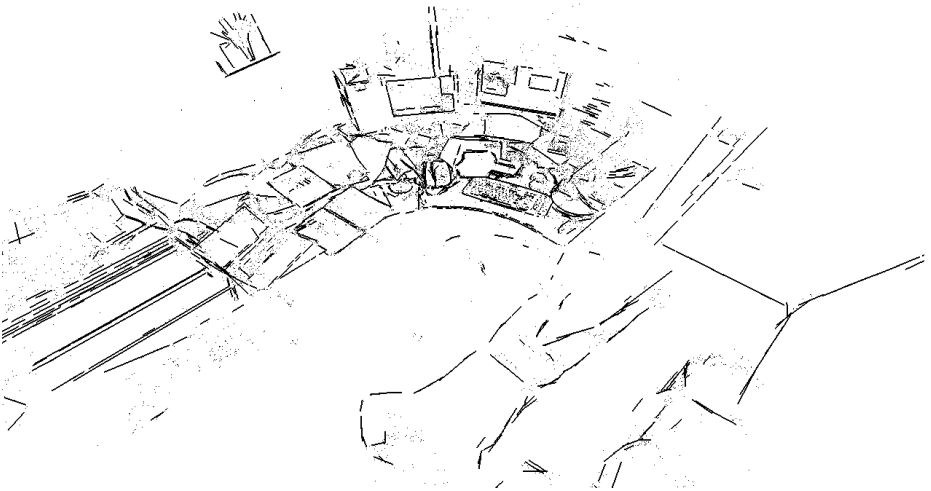
Fig. 4. A 3D map of an office scene with 9400 point features, 1800 edgelets and 250 keyframes. Some structure is clearly visible, including a door-frame, cabinet, resting researcher and a desk with some computer screens.
