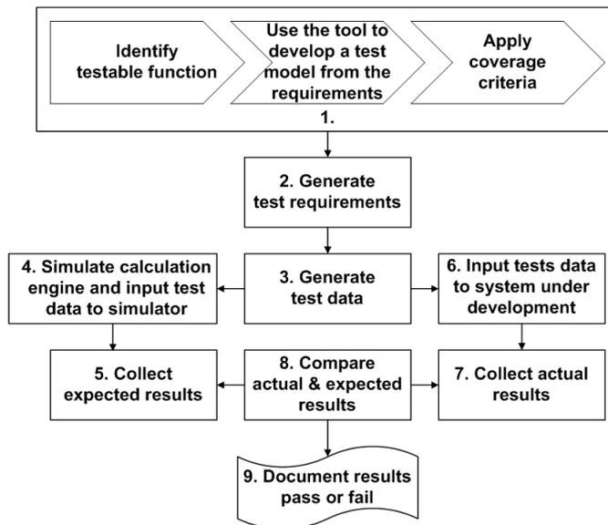
**Fig. 1** Modeling process to test calculation engines
