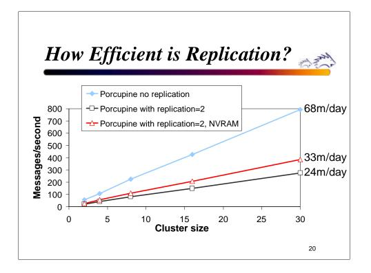
So we pretended that we have such hardware and simply removed synchronous disk flushing from the disk logging routines. We get this red line. This line still scales perfectly, and in addition, its performance is exactly what we expected, the half of the baseline case. So, to summarize, this graph shows that our replication algorithm is scalable, and is very efficient.
