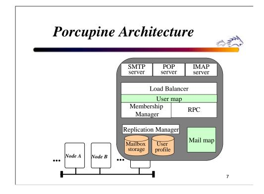
The picture shows the main components of the system. Porcupine consists of a set of nodes connected by a fast network. Because Porcupine is functionally homogeneous, all the nodes run the identical set of software.
