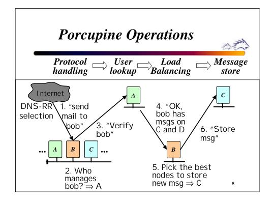
Now, I want to show a birds-eye view of how P works. This picture shows the steps performed during mail delivery. A client somewhere in the Inet chooses a node to contact using some naming mechanism such as DNSRR. Because of functional homogeneity, the client can in fact pick any node, but in this example, lets suppose it picked B. The client lets B know that it wants to send a msg to bob.
