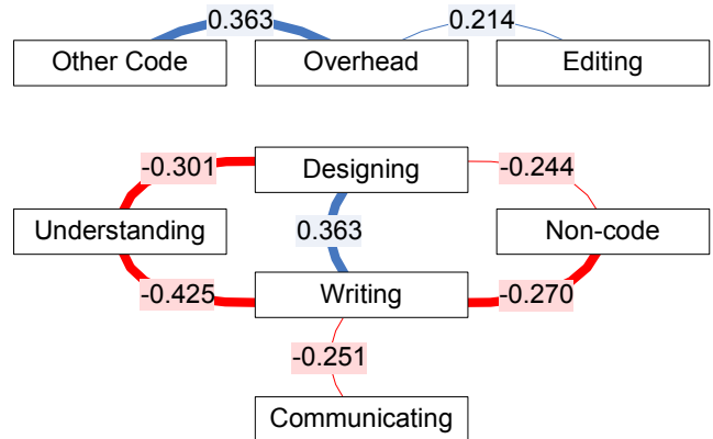
Figure 3. Statistically significant correlations between time spent on each activity. Negative numbers indicate inverse relationships. (Spearman's rho, thin lines for p < 0.05 , thick lines for p < 0.01 , n = 104 .)
