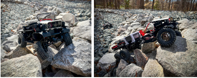
Fig. 7: Outdoor Demonstration: V4W’s right front wheel suspends in the air (left) and V6W climbs a steeper rock pile than the indoor testbed.
