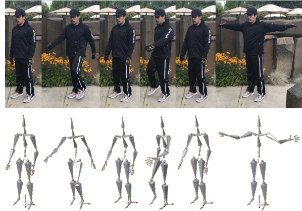
Fig. 1: Our system enables pose tracking over the long term with wearable sensors integrated into everyday clothing.
