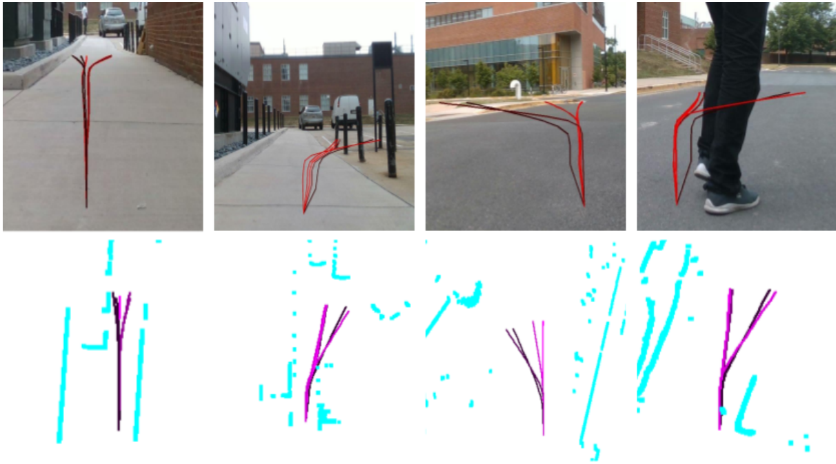
Fig. 5: Trajectory Confidence: The top row shows the camera view of the generated trajectories and the bottom row shows the bird-eye-view of the trajectories. The Cyan color represents the obstacles detected from the middle channel of the 3D Lidar.
