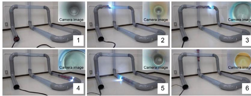
Fig. 11. AIRO-2 navigating through 8m's winding pipe.
