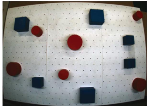
Fig. 9. AIKO-Pegboard consists of a reconfigurable modular obstacle course [17].
