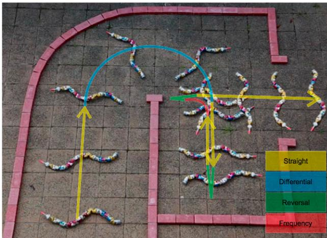
**Fig. 3.** CMU Modular Snake traversing CMU-MS-Mockup2, which is representative of all testbeds constructed to delimit different types of restricted maneuverability spaces [9–11].
