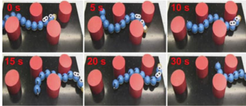
Fig. 7. Kulko traversing through Kulko-Pegboard [15].
