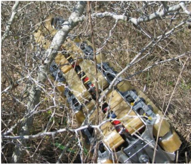
**Fig. 10.** OmniTread traversing dense underbrush. Rather than being stuck by the branches touching the robot from all directions, powered tracks around the snake robot provide extra propulsion against the environment.
