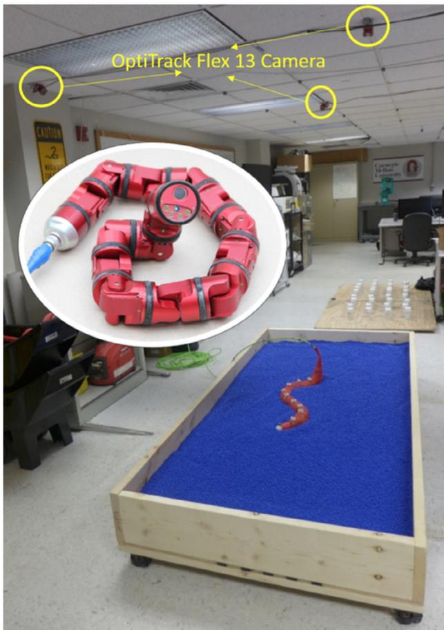
**Fig. 5.** CMU SEA Snake swimming through CMU-SEA-BB (pool) testbed filled with simulated granular material. This is the only testbed found to emulate environments with  $E_{cd}/A_{cd} \leq 1$  [22].
