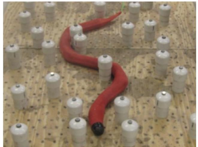
**Fig. 4.** CMU SEA Snake slithering through CMU-SEA-Pegboard with reconfigurable peg pattern through mounting holes, which is a typical representation of all pegboard-type testbeds used in [6,15,17,25].
