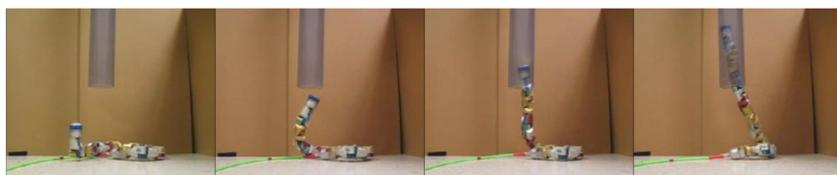
**Fig. 1.** CMU Modular Snake negotiating CMU-MS-Pipes testbed, which is representative of pipe testbeds in [7–9,16,18–20].
