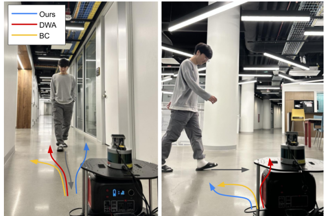
Fig. 1: Our approach (blue) demonstrates more social compliant than DWA (red) and BC (yellow) approaches in the frontal encountering scenario (left) and the intersection scenario (right).
