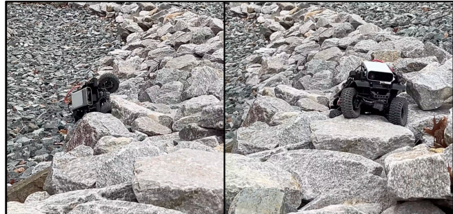
Fig. 6: Outdoor Mobility Demonstration: BC rolls over (left) and WM-VCT succeeds (right).
