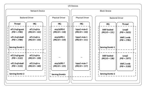
**Figure 7.** Identification of related workers in the driver domain for each domain. In this example, a network device and a block device are allocated to both DomU-1 and DomU-2. Thread "vif1.0-q0-guest", with PID = 2783, serves the virtual network device in DomU-1. IRQ "enp2s0f0-0", with IRQ ID = 118, serves the physical network device in the driver domain. Those workers can be grouped by the domains they serve: 1) serving only DomU-1; 2) serving only DomU-2; and 3) serving both.
