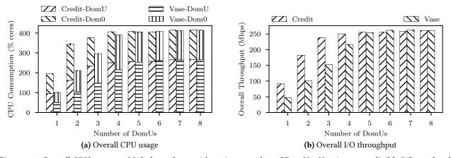
**Figure 10.** Overall CPU usage and I/O throughput with various number of DomUs. *Vase* incurs negligible I/O overhead when CPU is saturated (DomUs > 4). When it is not, *Vase* accurately limits DomU's CPU usage, and hence their I/O throughput.
