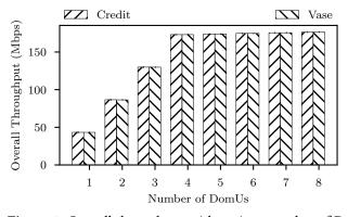
**Figure 9.** Overall throughput with various number of DomUs running CPU intensive workloads, which shows *VASE System* introduces negligible overhead to CPU throughput.
