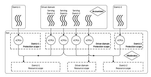
**Figure 6.** The overall design of *VASE System*. The resource scope of each domain is defined by the actual resource consumption of that domain as opposed to falsely defined by the protection scope. The existing vCPU abstraction is used as resource container to isolate and encapsulate the offloaded workload. *VASE System* enables such resource scope using two major components: 1) An *Accountant* component in the driver domain; and 2) A *Moderator* component in the Xen hypervisor.
