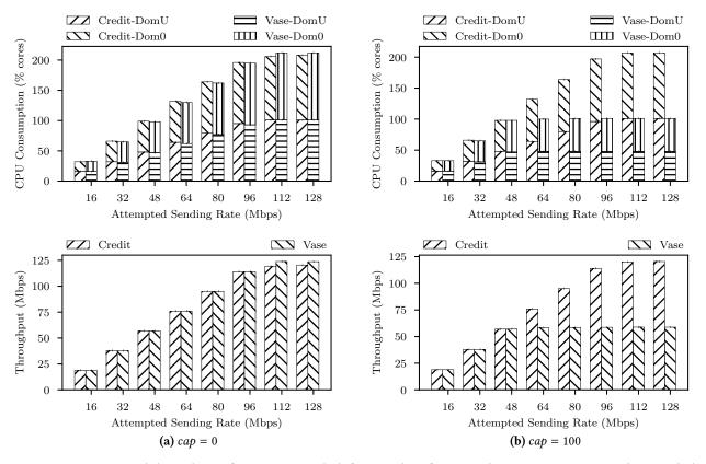
**Figure 8.** CPU usage and throughput of one DomU with different values for *cap*. When *VASE System* is implemented, the total CPU consumption of DomU is precisely limited by the given cap values. On the contrary, it can reach up to twice the allocated amount in the original setting. Thus, *VASE System* accurately enforce the resource consumption limit of DomUs.
