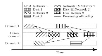
**Figure 1.** Illustration of software-based I/O virtualization: much of I/O processing is offloaded to the driver domain, which is not accounted to its source domain (domain-1/domain-2). Such offloading processing: 1) is asynchronous with processing in the source domain; and 2) interleaves with each other in the driver domain.
