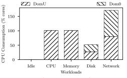
**Figure 3.** System-wide CPU usage with one DomU running various workloads. The total CPU usage reaches more than 170% (of a CPU core) in case of I/O intensive workloads, exceeding the amount of 100% that is allocated to the DomU. The exceeding part is "stolen" from other domains.
