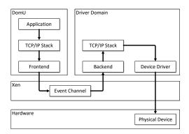
**Figure 2.** The path of sending a packet in Xen [10]. In the split driver model, a large portion of I/O processing happens in the driver domain, consuming a significant amount of CPU resource on behalf of the DomUs.
