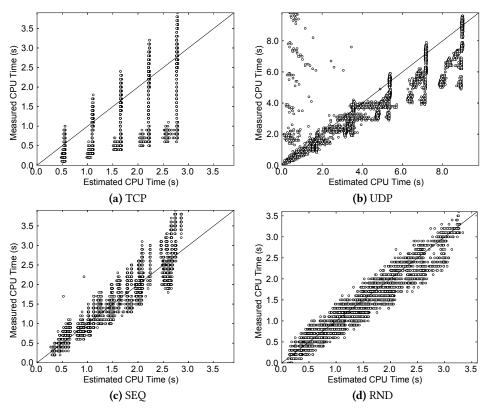
**Figure 4.** The true and estimated CPU time of the driver domain when running I/O intensive workloads. The diagonal line represents an accurate estimation. The estimation approach yields up to 79% errors for network and 50% for disk.
