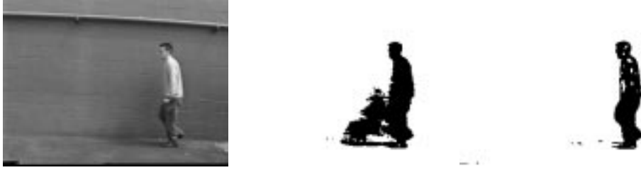
FIG. 2. Example of background subtraction. Left: Color image from sequence. Center: Connected components using RGB background model. Right: Connected components using combined chromaticity and gradient background model.
