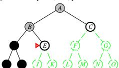
Expand deepest unexpanded node
