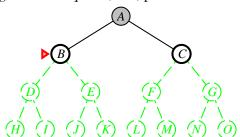
Expand deepest unexpanded node
