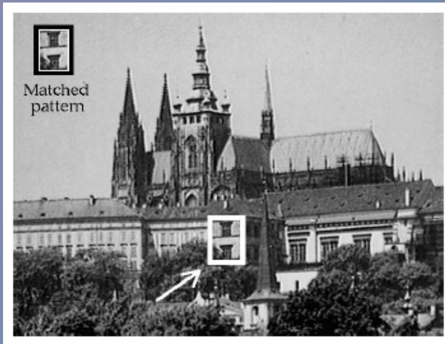
Figure 6.52: Segmentation by matching; matched pattern and location of the best match.
