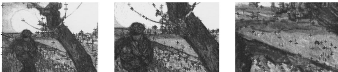
Figure 11. Interest points detected on the images of Fig. 10 using the improved version of Harris. There are 317, 399 and 300 points detected in the left, middle and right images, respectively. The repeatability rate between the left and middle images is 54% and between the left and right images 1% for a localization error \epsilon of 1.5 pixels.
