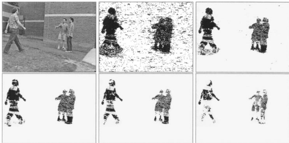
FIG. 4. The effect of varying the threshold on color-based subtraction. From top left: original image (same as fourth frame in Fig. 1) and results of thresholding at 1, 2, 3, 5, and 10 standard deviations.
