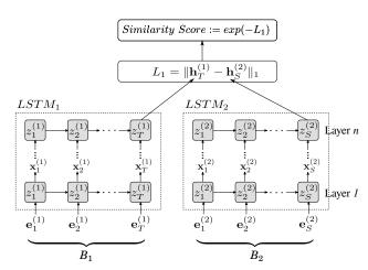
Fig. 5: Neural network-based basic-block embedding model. Each shaded box is an LSTM cell.
