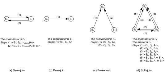
Only the data transmission steps are shown. Each step follows the form: <sender, receiver, data>.
